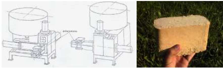
Fig. 2: a) Single-piston press and its product b) Multi-piston press and its product
